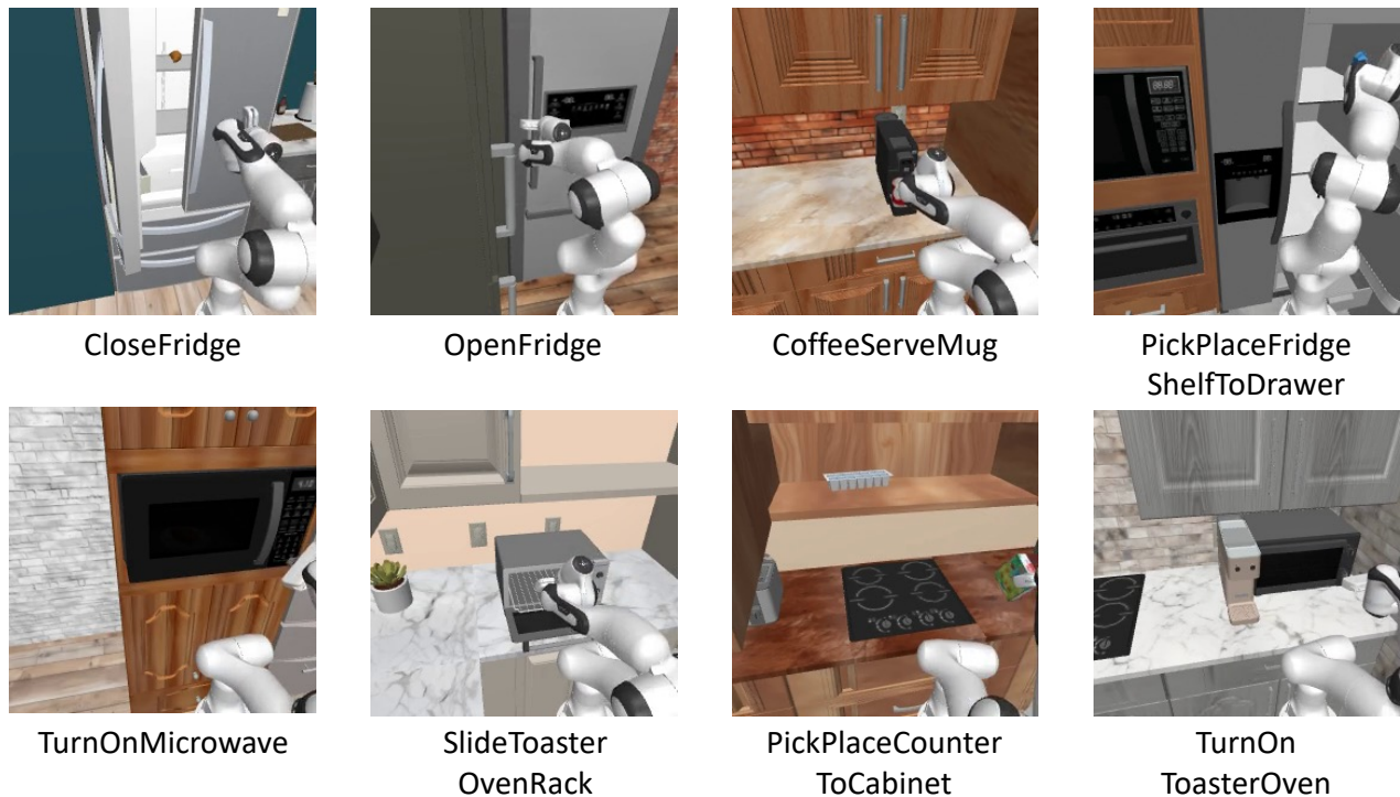
Figure 8: RoboCasa365 simulation examples. Example evaluation scenes from the 8 RoboCasa365 tasks used in our simulated experiments. The benchmark randomizes scene layouts, object instances, and initial configurations across rollouts, emphasizing policy generalization rather than memorization of a fixed scene.
